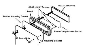
Mount the DLXT light(s) on the bracket as shown above. Use the two #6-32 x 5/16" screws through the back of the mounting bracket as shown. Secure the screws using the two #6 acorn nuts. Repeat for additional lights, if applicable.
